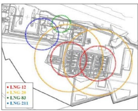
Golden Pass LNG Liquefaction Export Project – LNG Flammable Vapor Dispersion Exclusion Zones
